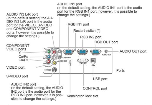
**NOTE** (\*) About Restart switch: This projector is controlled by an internal microprocessor. Under certain exceptional circumstances, the projector may not operate correctly and the microprocessor will need to be reset. In such a case, please push the Restart switch by using a cocktail stick or similar, and before turning on again, make the projector cool down at least 10 minutes without operating. Only push the Restart switch in these exceptional instances.
